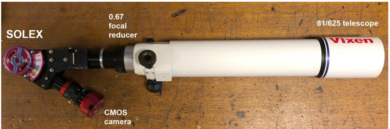
Figure 5: The Meudon SOLEX: it uses a 625 mm focal length refractor; the diameter of the solar image exceeds the 4.5 mm slit of the SOLEX and must be reduced. Therefore, we use a 0.67 x focal length reducer to have an equivalent focal length of 420 mm.
