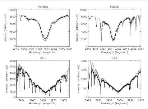
**Figure 3.**  $H\alpha$ ,  $H\beta$ , CaII H and CaII K line profiles near disk center (thick line) in comparison with atlas profiles, from Delbouille, Roland, and Neven (1973) (thin line). Sampling points are indicated by crosses.
