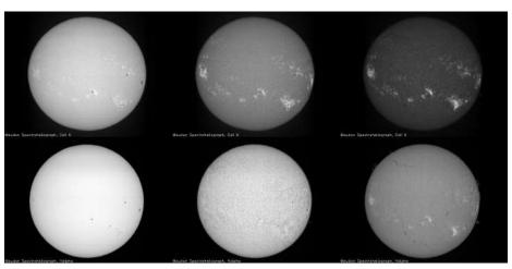
**Figure 5.** Example of images derived from profiles. Bottom:  $H\alpha$  -0.15 nm, -0.05 nm, center. Top: CaII K -0.15 nm, -0.05 nm, center (tests of November 13, 2013)
