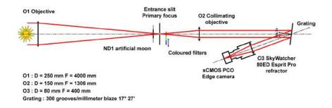
Figure 2. Optical design of the 2018 version of the spectroheliograh
